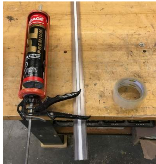
The supplies: LePage: PL Premium 3X & caulking gun, 3-foot hinge, packing tape (not pictured: a popsicle stick)
